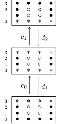
Figure 1: Jacobi iteration on a two-dimensional grid: ● = boundary cell, ○ = interior cell, \* = ghost cell
